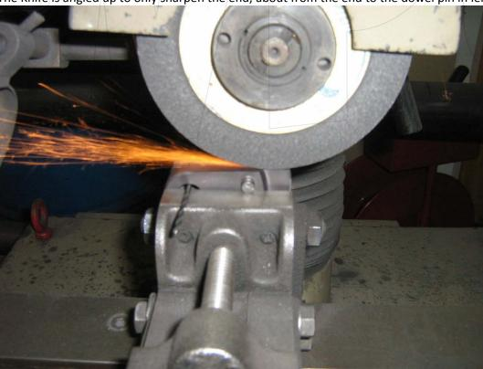
After this side is sharpened, the knife is stood on end and the cutting edge is placed level in the grinding machine.
