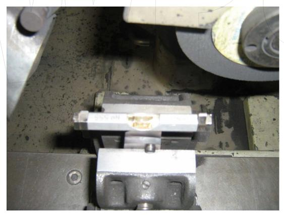
The entire length of the cutting face is then sharpened.
