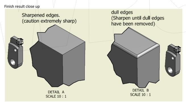
The finished knife should look polished where it is sharpened and shine more than the rest of the knife which will be a flat dark grey color. **The edges should be extremely sharp to properly function**.
